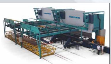
Ursviken's engineers develop and build highly efficient material handling systems that move large and heavy plates in and out of big press brakes at high speed.
