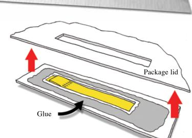
Persson's Handle applicator attaches glue to the top of the handle and mounts it on the inside of the package's lid.
