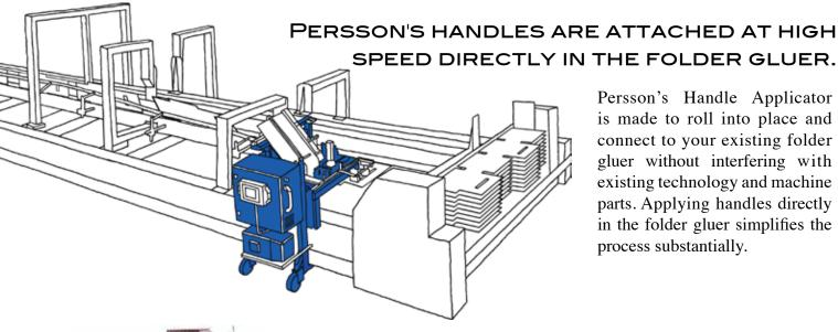
Persson's Handle Applicator is made to roll into place and connect to your existing folder gluer without interfering with existing technology and machine parts. Applying handles directly in the folder gluer simplifies the process substantially.
